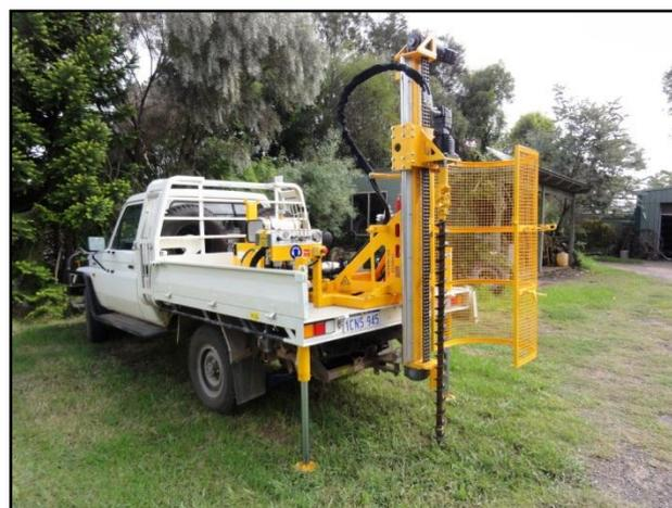
Figure 3: Helix Auger Rig will allow our team to sample a consistent soil horizon across areas of variable cover (up to max 20m). This will be used to identify drill targets on the southern extensions of the Tritton and Kurrajong VMS trends for testing in 2H12.
