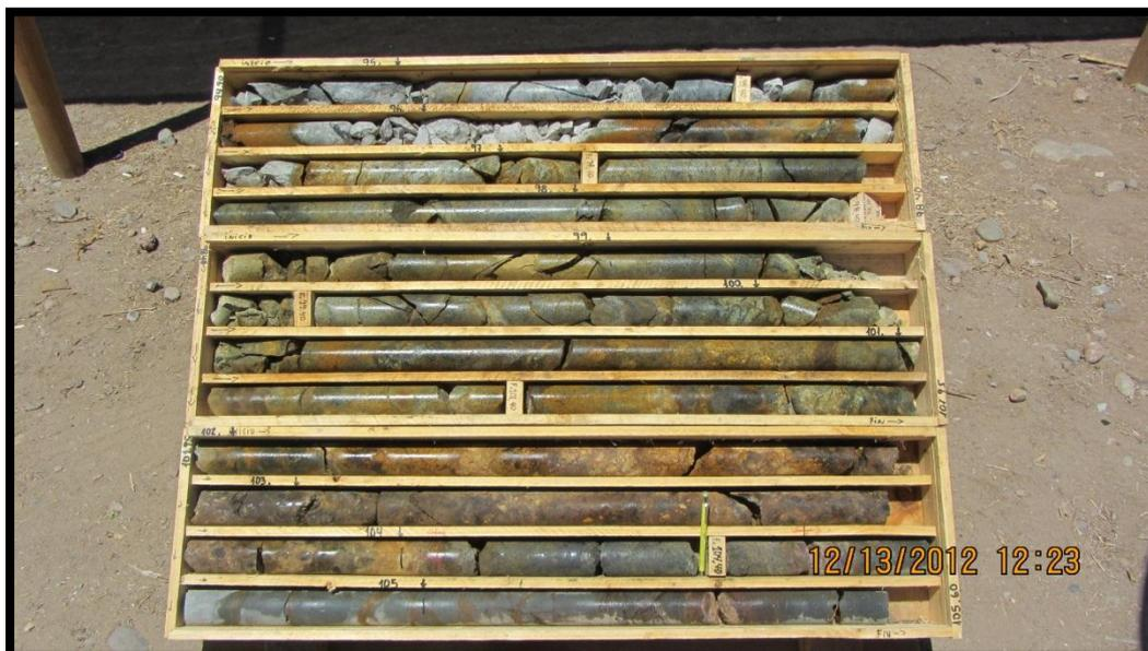
Copper mineralisation in core from approximately 95m to 104.5m in DDHHU-001 (bottom 50% of mineralised intercept)
