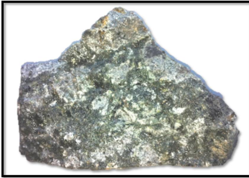
Figure 1: Brecciated Dacitic Porphyry with disseminated chalcopyrite and chalcocite from the base of the Carmelita workings (~50m below surface) on the eastern edge of Target 1. Sample assayed 3.1% Cu, 0.1g/t Au, 11g/t Ag and 200ppm Mo (Refer to ASX announcement dated 30 January 2015).
