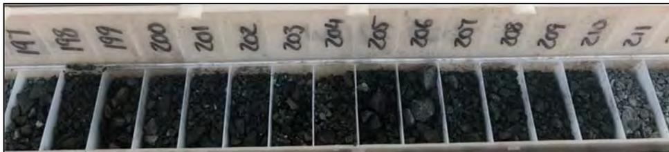
*Figure 1: Zone of massive and semi-massive sulphide in a silica-rich unit (probable exhalite) in MURC002; zone correlates well with the DHEM modelled plate position.*
